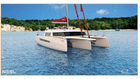
Builder: NEEL Trimarans Architect: Marc Lombard Yacht Design Length: 52'2" (15.9 m) Beam: 28'10" (8.8 m) Draft: 6'3" (1.9 m) Air draft: 79'1" (24.1 m) aluminum mast 81'4" (24.8 m) carbon mast Light displacement: 27,780 lbs (12.6 t) Laden displacement: 42,990 lbs (19.5 t) Mainsail: 1,022/1,098 sq ft (95/102 m<sup>2</sup>) Genoa: 764 sq ft (71 m<sup>2</sup>) Staysail: 344 sq ft (32 m<sup>2</sup>) Water: 158 US gal (600 l) Fuel: 185 US gal (700 l) Engine: 110 HP
