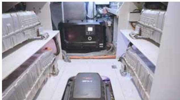
Engine room space is mostly given over to batteries
