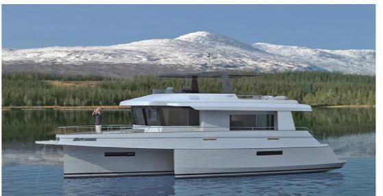
**Top:** the super-wide platform of a Neel tri gives you considerably more living space at anchor than even a cat of similar length. The central hull improves weight distribution, allowing all heavy equipment and systems to be low down and centrally located. **Above:** Neel's new Leen power tris have the same core values – and designer Bernard Nivelt owns one...
